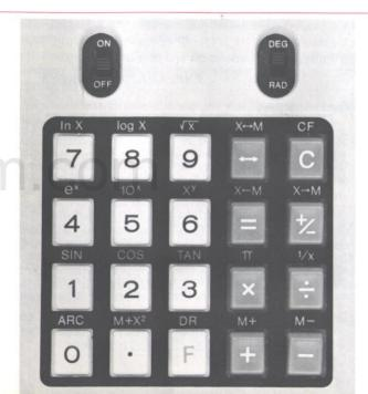
The Rockwell 202 Slide Rule has algebraic logic. This means it calculates the way you think. It also has a unique "second function" key that allows each key to have two separate uses. The first use, represented in this manual by a , is identified on the keytop; the second use, represented by ( ), is identified above the keytop. The following explanation will help you understand the operation and uses of each key.
